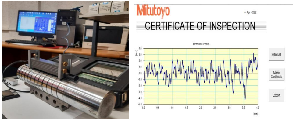
Fig3: Measurement of Surface roughness and theoretical results
