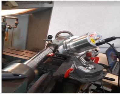
Fig2.1 Keller Cella Cast measuring temperatures during the turning process.
